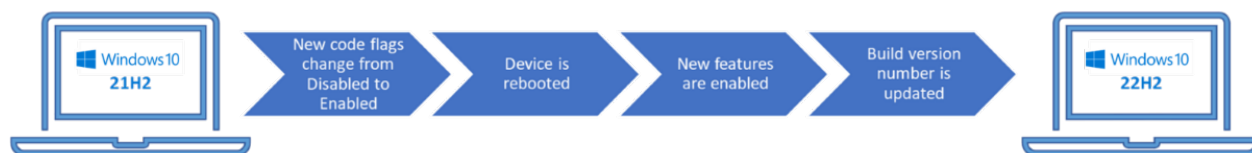
Figure 4. The four stages of an upgrade from one version to another: New code flags change from Disabled to Enabled, device is rebooted, new features are enabled, and build version number is updated.
